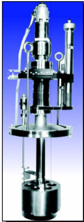
A full line of MBE Sample Manipulators and Preparation Stages are available for wafers from 1" to 8" in diameter. All have rotational capability, XYZ motion and heating to 1200 °C. A wide range of heating elements and thermocouple types are offered, with an optional built-in master shutter.
